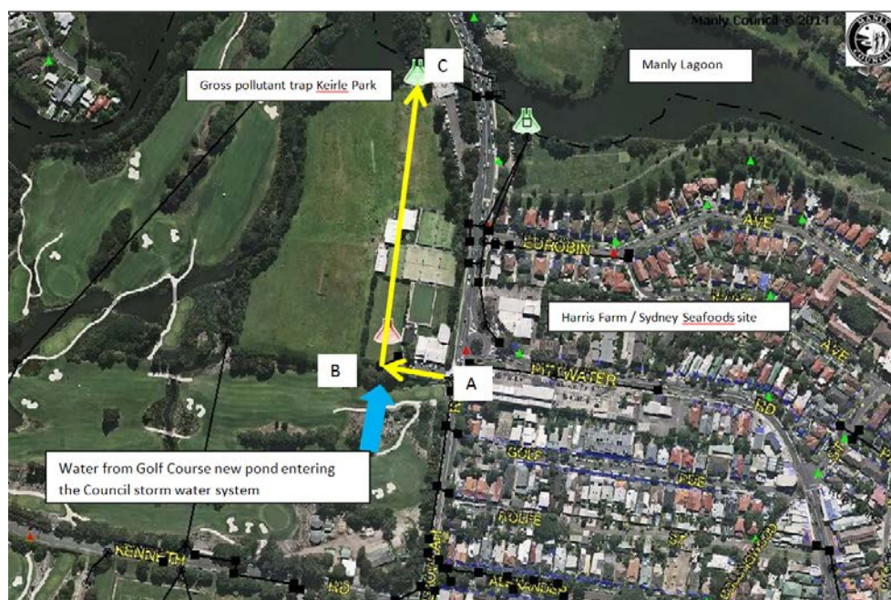
Figure 1.0 Aerial view of the flooding affected area The drainage line shown in yellow above extends from Balgowlah Rd and discharges water through a series of gross pollutant traps to the Manly lagoon
