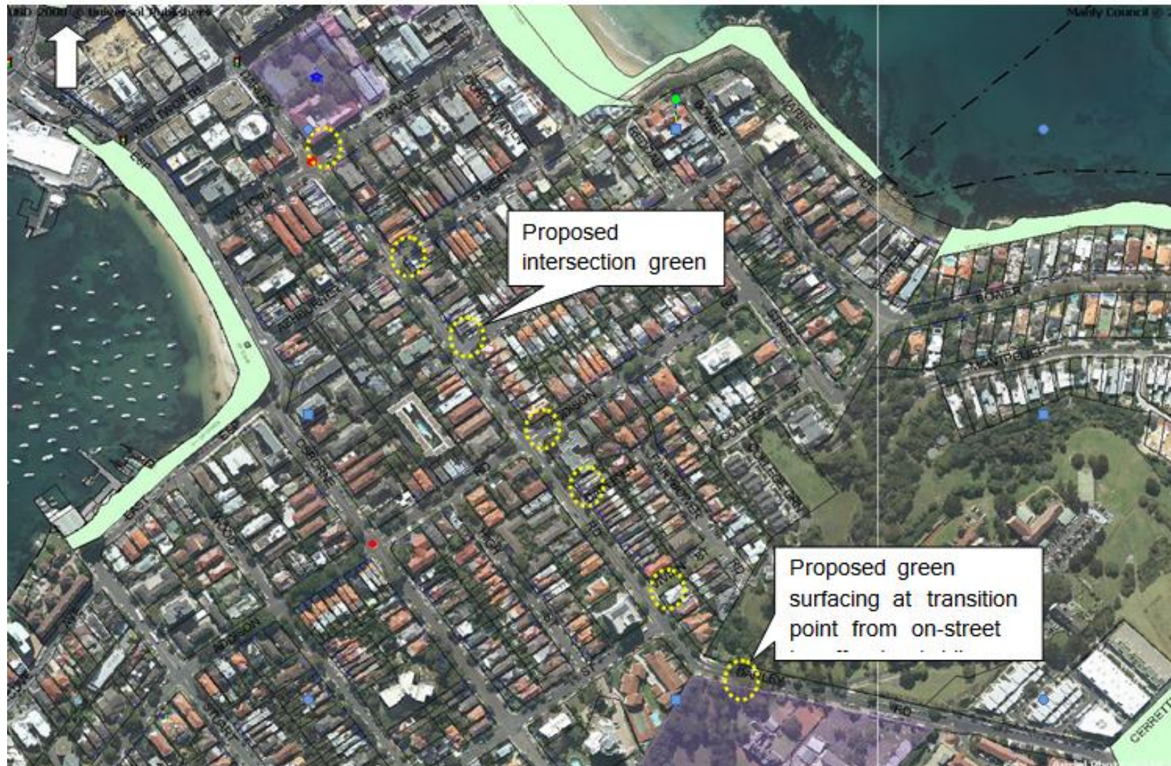
Figure 1– Proposed green surfacing along Darley Road
